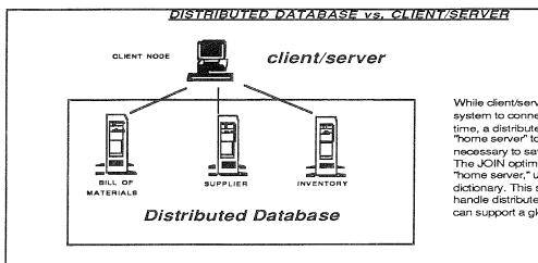
While client/server requires the client system to connect to one server at a time, a distributed DBMS enables the "home server" to call other servers as necessary to satisfy the client request. The JOIN optimization is handled by the "home server," using the system dictionary. This server node can handle distributed transactions and can support a global schema view.
