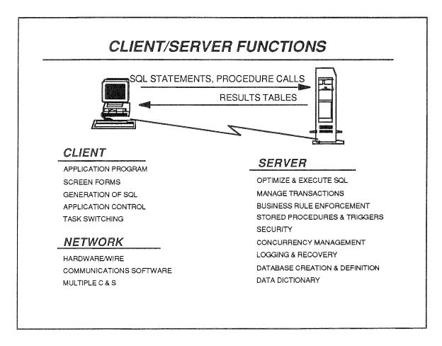
have appropriate interface cards in both the client and server machines. The communications software typically handles different types of transportation protocols, such as SPX/IPX, LU6.2, and TCP/IP. Most network environments provide support for multiple clients and servers.
